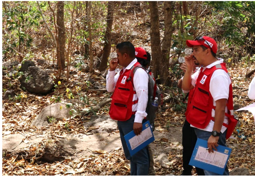
Illustration 7: Data collection of slope of rockfall events in Honduras using a clinometer. Source: SRC.
