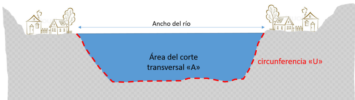
Illustration 10: Schematic cross profile. The blue area multiplied by the runoff velocity equals the maximum discharge capacity of the river. The circumference "U" for the determination of the hydraulic radius is presented in dashed red. Source: SRC.
