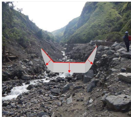
Illustration 11: Segmentation of the torrent into sections morphologically uniform (left). For each section, a cross-section is established for which the erodible depth is defined (right. Grey areas).
