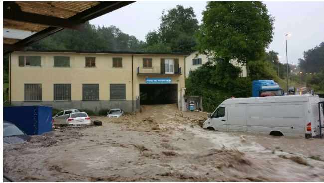
Illustration 11: Medium intensity flood. Vehicles and persons may be swept away due to flow velocity and flow height.
