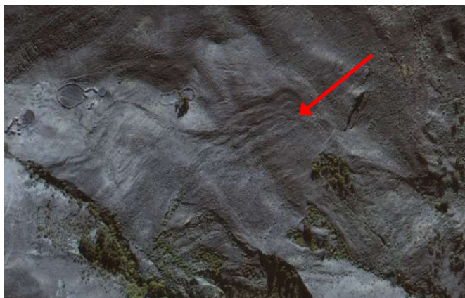
Illustration 10: Undulating surface (arrow) indicating a permanent landslide. Watercourses are usually missing in the area of the sliding body due to the continuous deformation of the surface. Source: GEOTEST AG.
